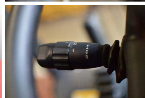
Ergonomic instrument panel: integrated handle switch, ratchet type hand brake and integrated electro-hydraulic reversing handle
