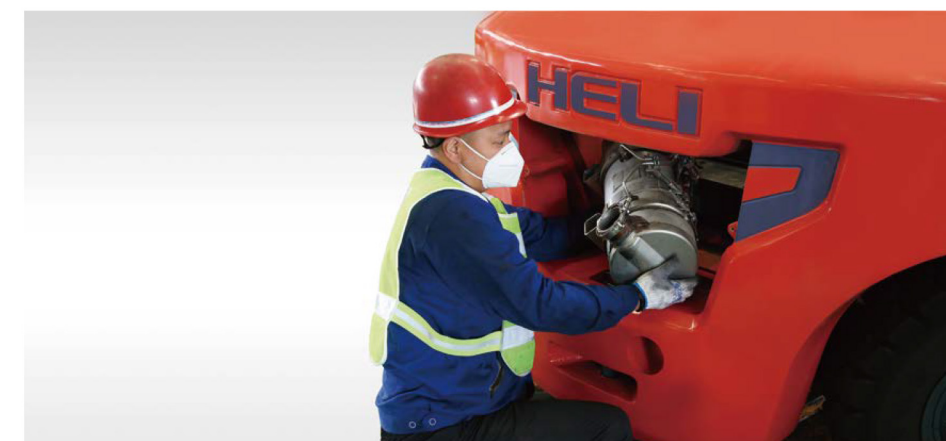
Easy to remove from exhaust aftertreatment Facilitates regular maintenance
