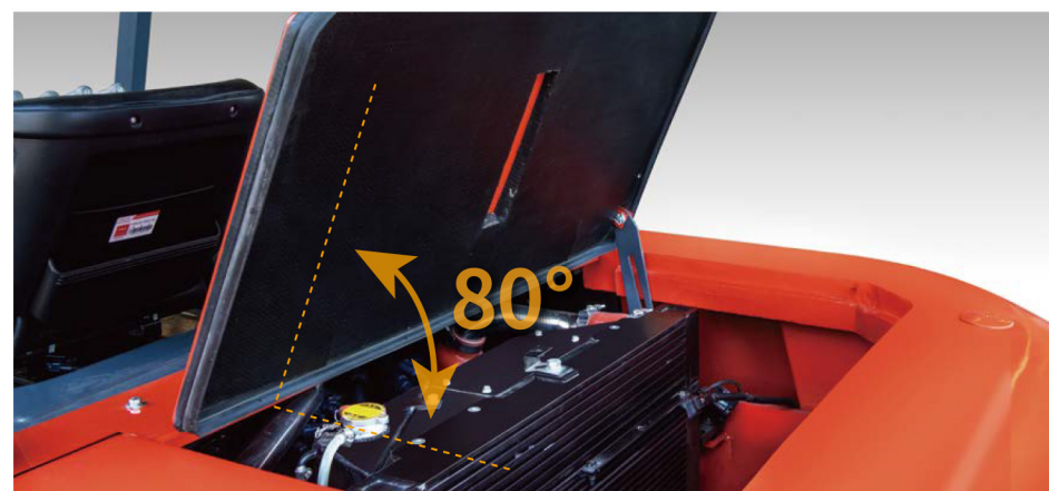
Radiator cover with supporting rod can open to 80 degrees. It is convenient to check
