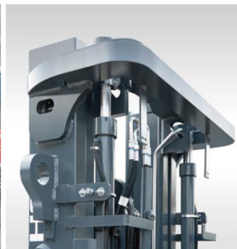
Reinforced beams for increased stiffness and strength
